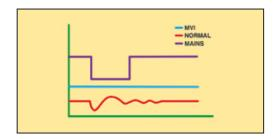
The JOFRA ATC-320 and ATC-650 calibrators employ the MVI, thus avoiding such stability problems. The MVI circuitry continuously monitors the supply voltage and ensures a constant energy flow to the heating elements. The JOFRA ATC-156 and ATC-157 models run on stabilized DC voltage and thus do not need the MVI circuitry.
