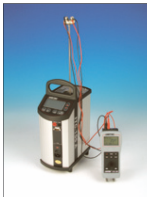
CSC200 as RTD input with an ITC
