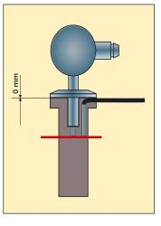
Below you see the custom insert and STS-102 A reference sensor placed in a JOFRA ATC-156 B dry-block calibrator. On the right, the sanitary sensor has been fitted into the insert and is ready for calibration. Note that the design makes room for the reference sensor cable.
