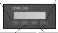
The MENU/ENTER key includes intelligent prompts that guide the user through setup and operation. This key allows the user to specify measuring units, resolution, sensor identification, and coefficients.
