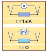
True Ohm Measurement is a proven method to achieve accurate compensation for errors induced by thermal effects.
