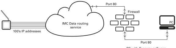
PC with Synergy software will call for data using Port 80
