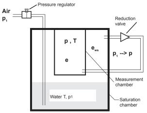
Schematic Illustration of a Two-pressure Reactor
